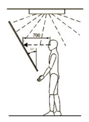
Panel evaluation should take place under a diffuse and fixed light source that illuminates the surface uniformly. This can be sunlight or adequate artificial lighting (between 2000-5000 lux). The approximate distance between the assessed surface and light source should be 1,5m. Surface defects will only be acknowledged if they are larger than 0,8mm² and visible from a distance of 0,7m at a viewing angle of approximately 45°.
