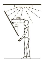
Panel evaluation should take place under a diffuse and fixed light source that illuminates the surface uniformly. This can be sunlight or adequate artificial lighting (between 2000-5000 lux). The approximate distance between the assessed surface and light source should be 1,5m. Surface defects will only be acknowledged if they are larger than 0,8mm² and visible from a distance of 0,7m at a viewing angle of approximately 45°.
